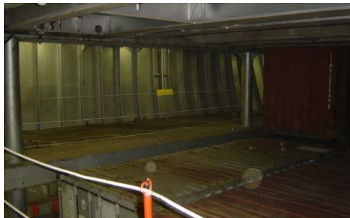
Fig 212 - Typical 'tween deck space
